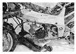
• Remove the engine mounting bolts (A), (C).
